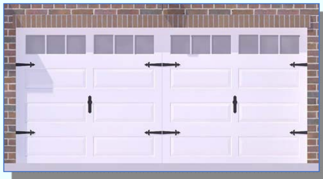
2.2 Single, 16-foot-wide garage door to mimic 2-individual doors with style and hardware
