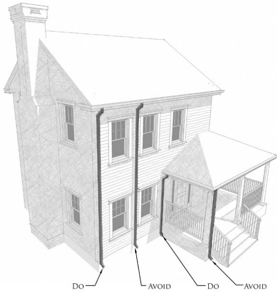
32.1 Downspouts should be located at interior or exterior corner. Downspouts in the middle of the facade should be avoided.
