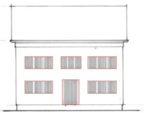
26.3 Use vertical proportions generally. Avoid horizontal windows unless they are composed of groups of square or vertical windows.
