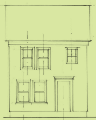
26.4 Misaligned window in a simple facade creates a sense of disorder on the elevation.
